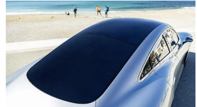
VISION EQXX with Solar roof by Fraunhofer ISE © Mercedes-Benz Group AG
